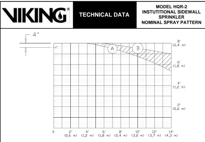
Typical side view of one half of the spray pattern produced by a Model Institutional Sidewall Sprinkler
